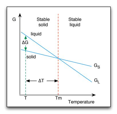
To get the solidification process started, the liquid phase must be undercooled, cooled to a temperature below the freezing point.
